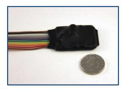
The input units are referred to as "universal" because they are more than simple switch interfaces. Each of the 8 inputs on a device may be assigned to be either a latching switch, a momentary contact, a  $3^{rd}$  Party Sensor with integral timeout, or a  $3^{rd}$  party sensor using system timeout. This enables the LightBox system to use a wide range of switches and  $3^{rd}$ party sensors to ensure the widest possible flexibility when designing a system for your application.
