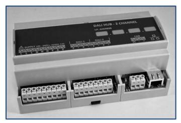
The DALI Hub is the first of a series of Hub units to be developed by MultiControls. The DALI Hub has been designed to work "out of the box" as a stand-alone 2 Channel DALI processor.
